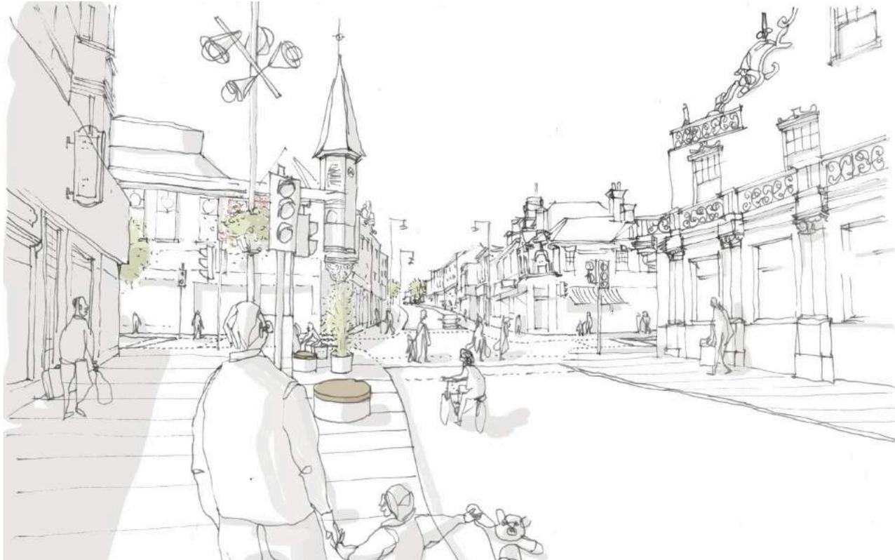
Figure 4.15: Sketch of High Street public realm proposals, looking west, showing footway build outs around junction, planters, seating objects and feature lighting
